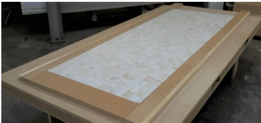
Image shows a door during construction with MDF frame and Balsa core
