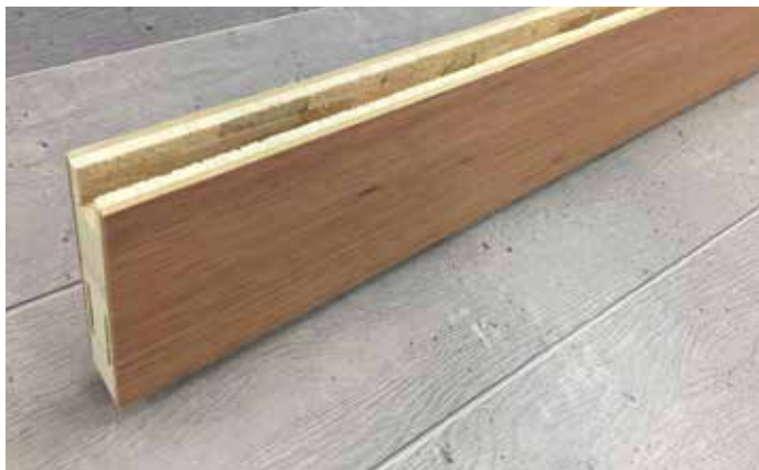
Installation method. Using a timber batten fixed to the ceiling the Ecolite beam is routed, fitted over the batten and secured by pins through the side of the beam into the batten.
